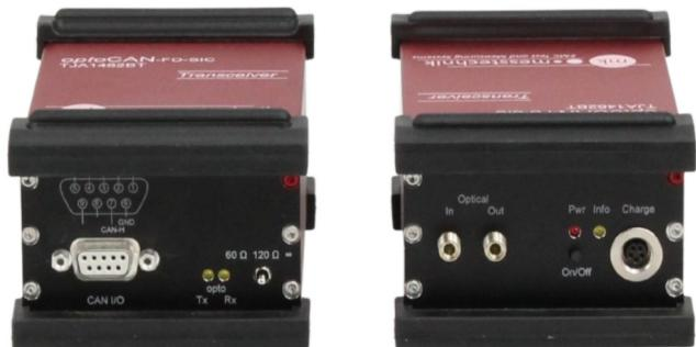
The system consists of two battery supplied transceivers connected to each other with an optical fiber. With the optical transmission and the shielded case, the system is well equipped for EMI and EME tests with automotive standards such as CISPR 25 class 5.
